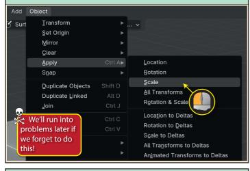
However, if we've set the Cube size solely by dragging to define the base and height, the Scale values will all remain at 1.0 irrespective of the Cube's actual dimensions.
