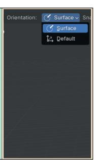
When set to **Surface**, the Local z-axis of the new Cube points in the same direction as the normal of the face it is positioned on.
