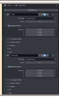
And if we change the parameter values in the second *Array modifier*, we can, for example, move the position of the latest copies.
