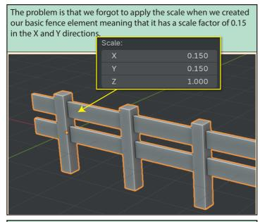
Those same scale factors have then been applied to any object that is assigned to the *Cap Head* and *End*. Hence, the two Cubes change to look like posts. To solve this problem we must first remove the *Cap Head* and *End* entries.
