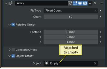
Now, if we rotate the **Empty** about its z-axis making the 60 copies rotate around 720°, we create out spiral staircase.
