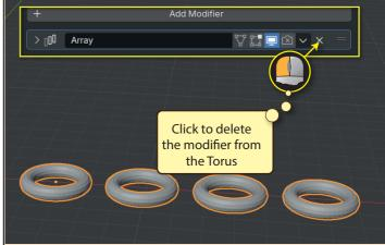
To demonstrate some of the uses of the Array modifier, we'll start by creating a metal chain. The first step is to create a Torus and shrink it in the Y direction.
