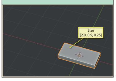
After applying the scaling, we'll move the Cube 1.7m along the x-axis.
