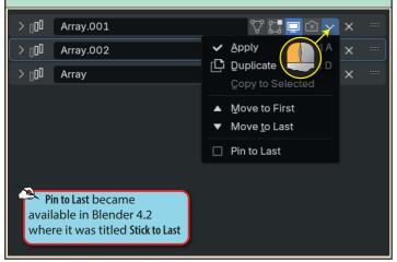
If we have more than one object selected when we apply a modifier, it will only be applied to the active object. However, once applied, the third option of the dropdown list, Copy to Selected, becomes activated.
