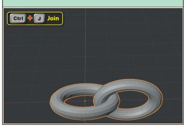
Now all we need to do is apply the *Array modifier*, adjust the **Relative Offset** in the X direction to around 0.8, and make as many copies as we require.
