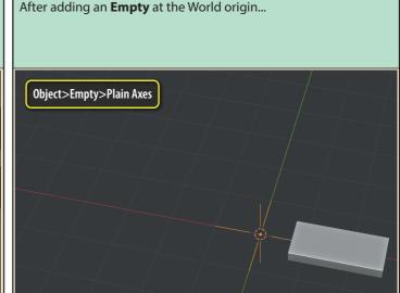
we'll select the Cube and apply an Array modifier setting the Count to 60 and the Relative Offsets to (0.0, 0.0, 1.0).
