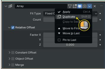
**Duplicate** creates another instance of the *Array modifier*. This copy applies the *Array modifier* to the results created by the first modifier.
