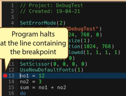
A screenshot of the code editor showing the same script as before. Line 13, which contains the breakpoint, is highlighted in blue. A yellow callout bubble points to this line with the text "Program halts at the line containing the breakpoint".
